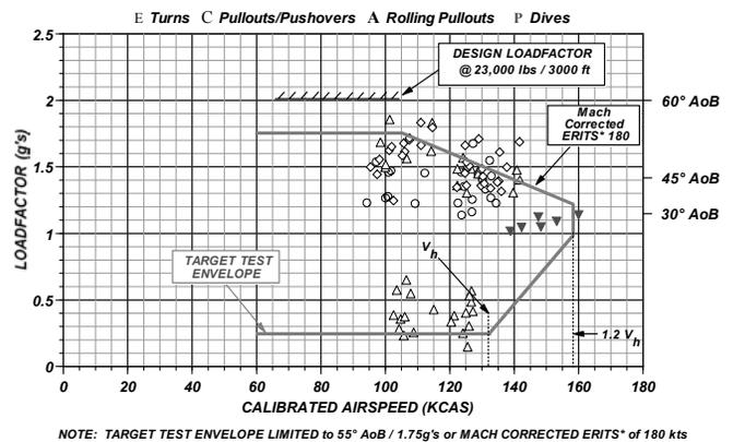
Figure 13 - Load factor vs Airspeed, Clean Config
