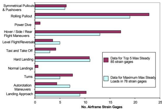
Figure 15 - Maneuvers Generating Highest Maximum Steady Loads for “High Reader” Airframe Strain Gages
