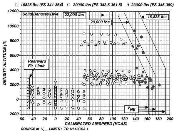
Figure 11 - Density Altitude vs Airspeed, Clean Config
