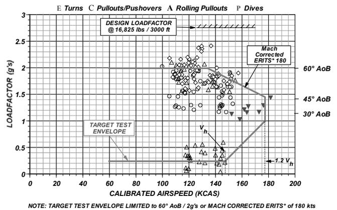
Figure 12 - Loadfactor vs Airspeed, Clean Config
