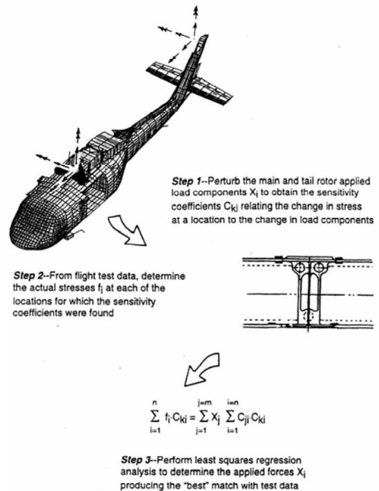
Figure 20 - Regression-Based “Correction” of NASTRAN External Loads
