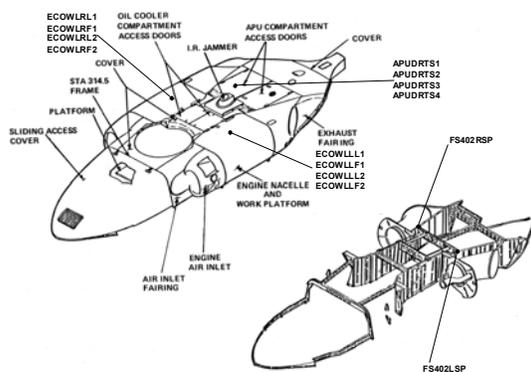
Figure 6 - Main Rotor Pylon Gage Locations
