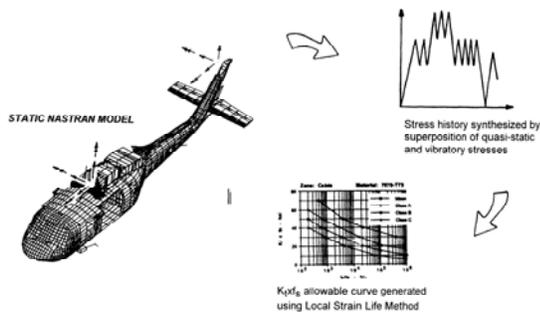
Figure 21 - FEM Fatigue Analysis Process
