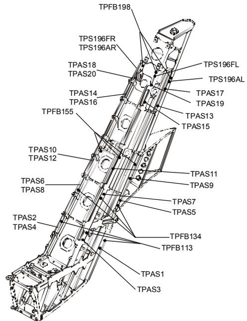
Figure 8 - Tail Pylon Gage Locations
