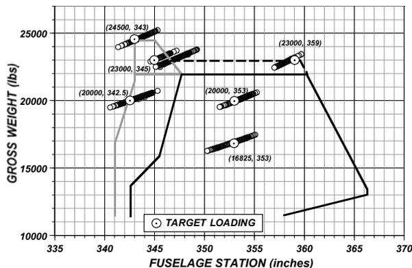
Figure 11 - ESSS Configuration Loadings
