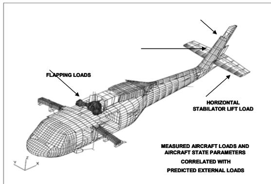
Figure 16 – Loads and Aircraft State Parameters to be Correlated with Flight Test Data
