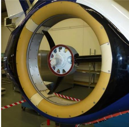
Figure 7: Integrated Fenestron® liner
