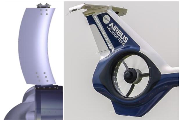
**Figure 3: Fenestron® stator design**
