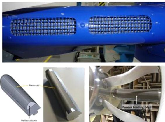
Figure 13: Special acoustic treatment at the leading edge of the drive shaft fairing
