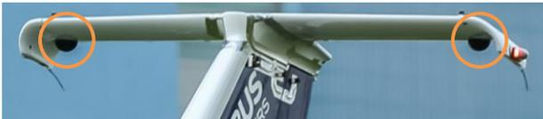
Figure 19: Right T-Tail surface microphone
