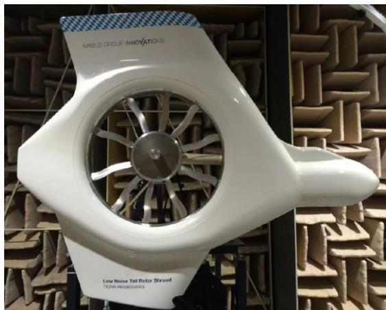
Figure 8: Fenestron® test bench at Airbus Group Innovations (Ottobrunn)
