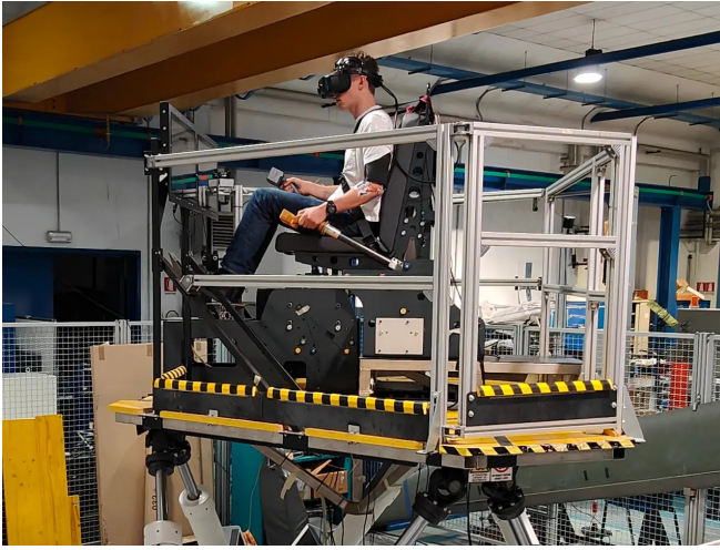
Figure 1. Photo of a participant in the pilot seat on the motion platform, wearing the Head-Mounted virtual reality display
