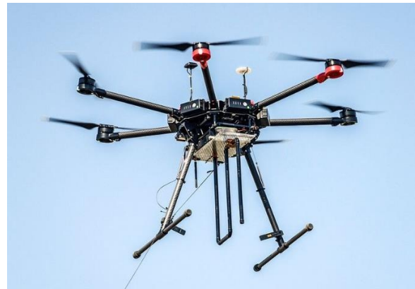
Figure 2: Top) FLIGHTLAB model of the UAV case study. Bottom) The DJI Matrice M600 [18], which is the case study UAV.
