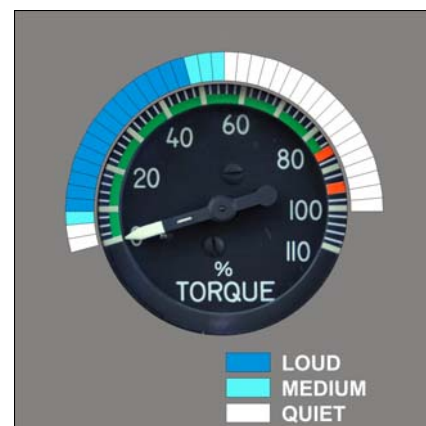
Fig. 16. Torque display extended as noise indicator to the pilot.
