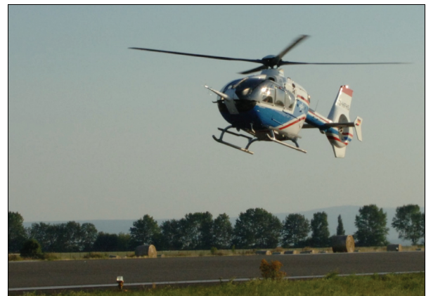
Fig. 1. EC135-FHS performing a flare with side-slip at Magdeburg-Cochstedt Airport during 2008 flight tests of noise abatement procedures.
