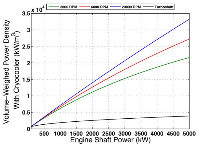
FIGURE 20 : HTS-motor with cryocooler  $Q_{P,V}$  (20K)
