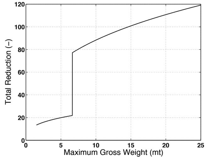
FIGURE 10 : Total reduction between engine output shaft and main rotor, based on survey data.
