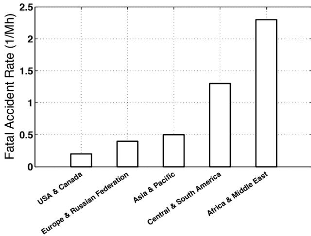
FIGURE 2 : Impact of geographic location of operations on accident rate per million of flight hours.
