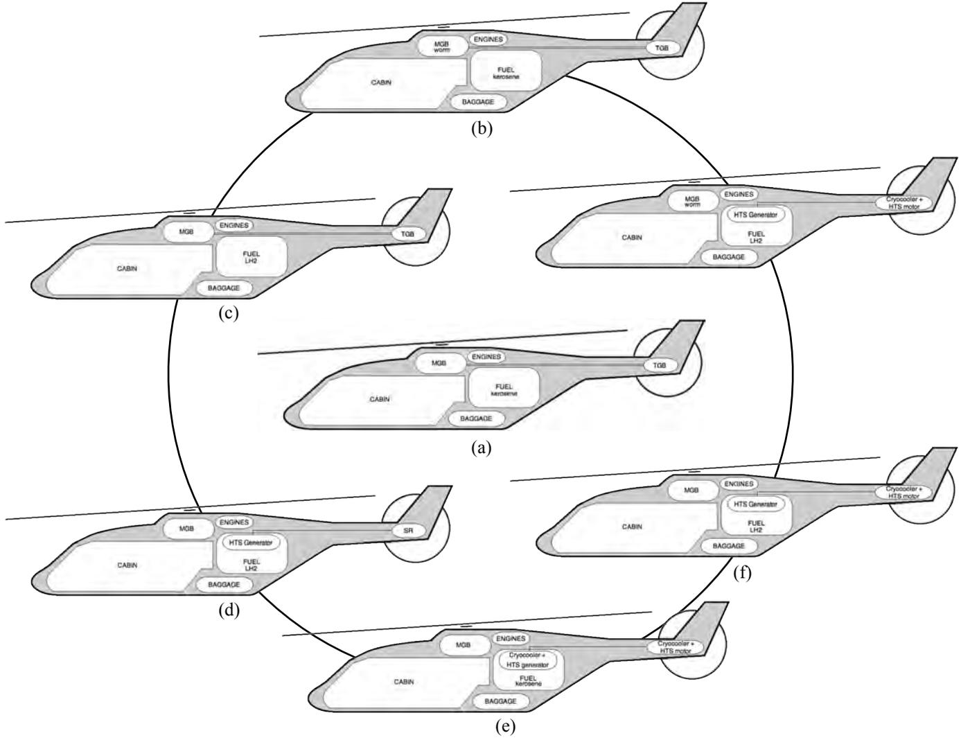
FIGURE 22 : The examined configurations
