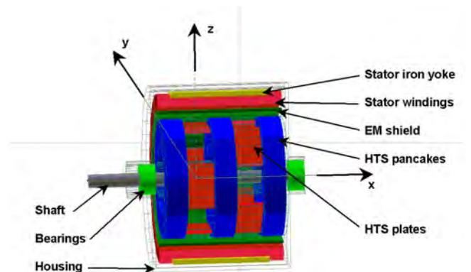
FIGURE 16 : HTS-motor using flux-trapping
