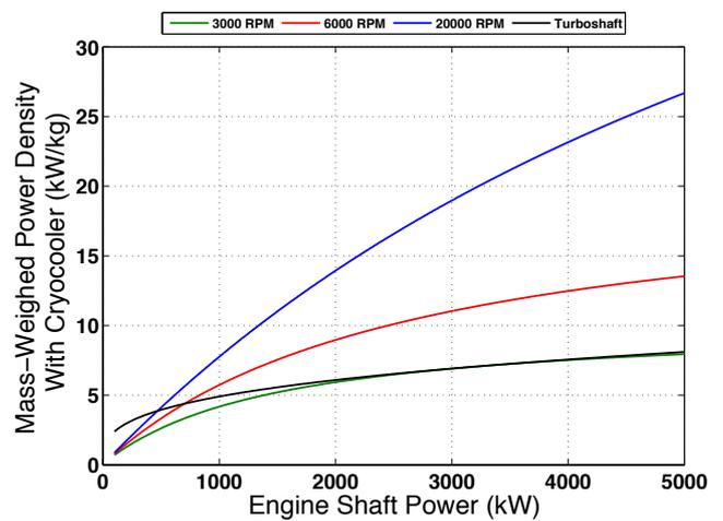
FIGURE 19 : HTS-motor with cryocooler  $Q_{P,m}$  (20K)
