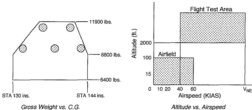
Figure 11 Flight Envelopes Tested
