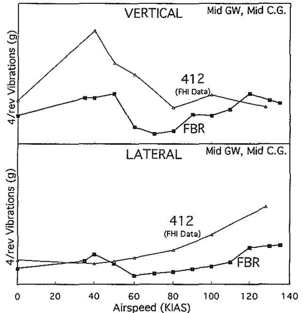
Figure 19 Vibration Levels at Pilot's Seat
