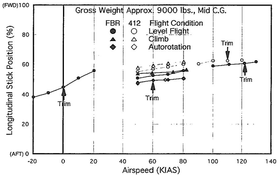
Figure 14 Static Longitudinal Stability
