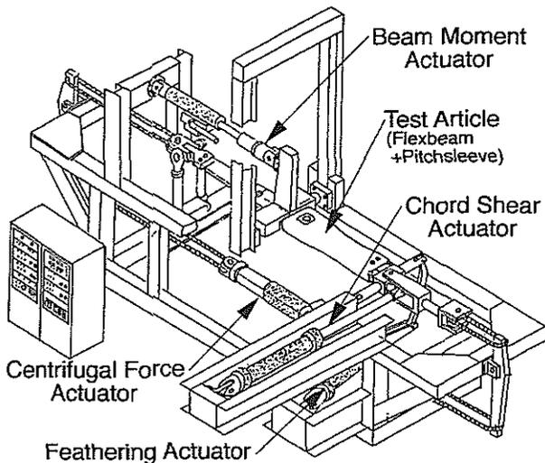
Figure 8 Hub Assembly Full-scale Test
