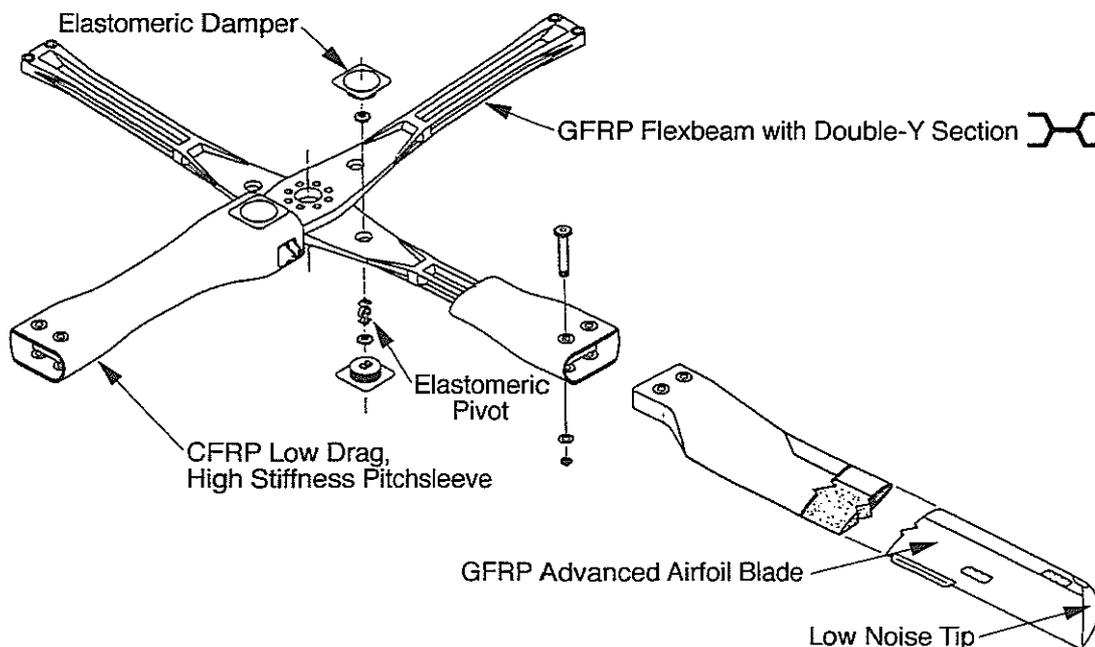
Figure 1 Outline of FBR Bearingless Main Rotor
