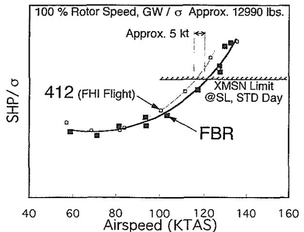
Figure 12 Level Flight Performance
