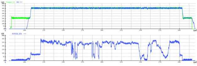
Figure 7: Nr control during flight after optimization
