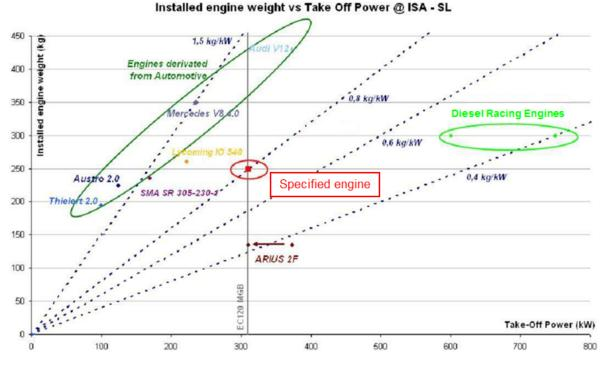
Figure 1: Installed mass-to-power ratio benchmark
