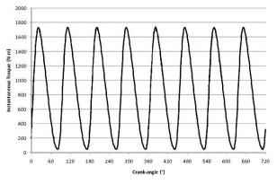
Figure 9: Instantaneous torque at crankshaft
