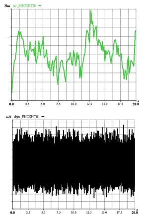
Figure 10: Static (green curve) and dynamic (black curve) part of torque at MGB inlet
