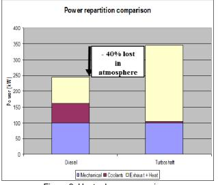
Figure 3: Heat release comparison
