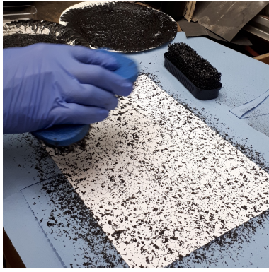
(a) speckle patten application with a soft plastic sponge
