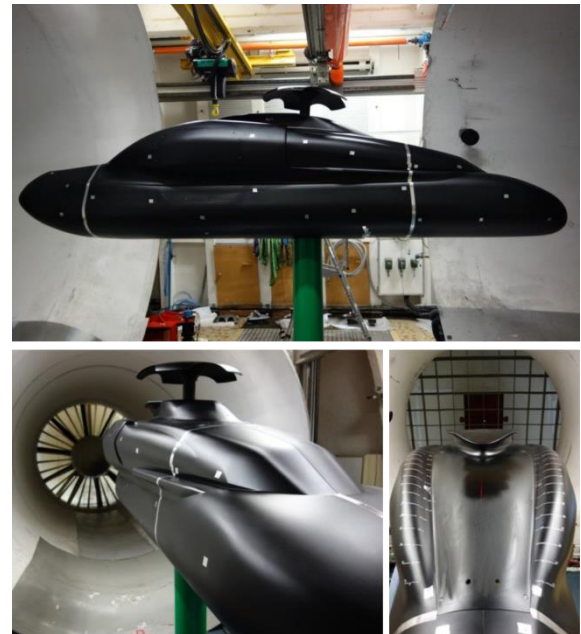
Figure 4 – Overview of the minibody configuration in the Marignane Wind-Tunnel facilities (here with a hub cap)
