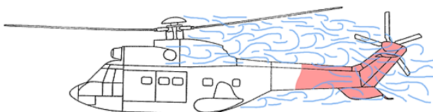
Figure 1 – Schematic illustration of the tail-shake phenomenon; in blue: wake; in red: impingement areas
