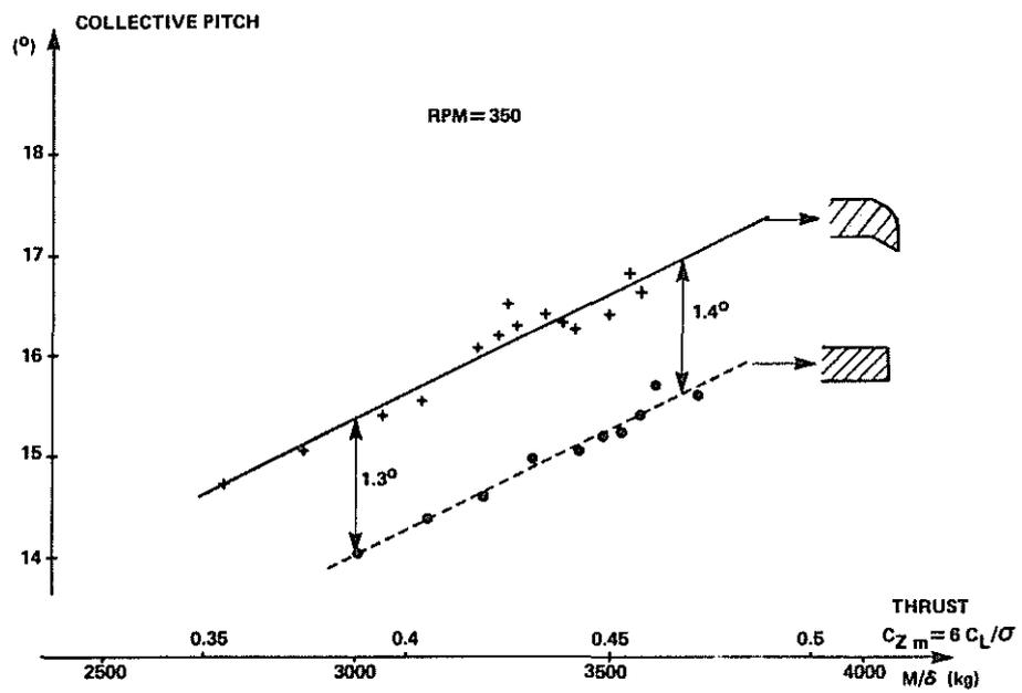
Fig. 8 COLLECTIVE PITCH AT BLADE ROOT IN HOVER
