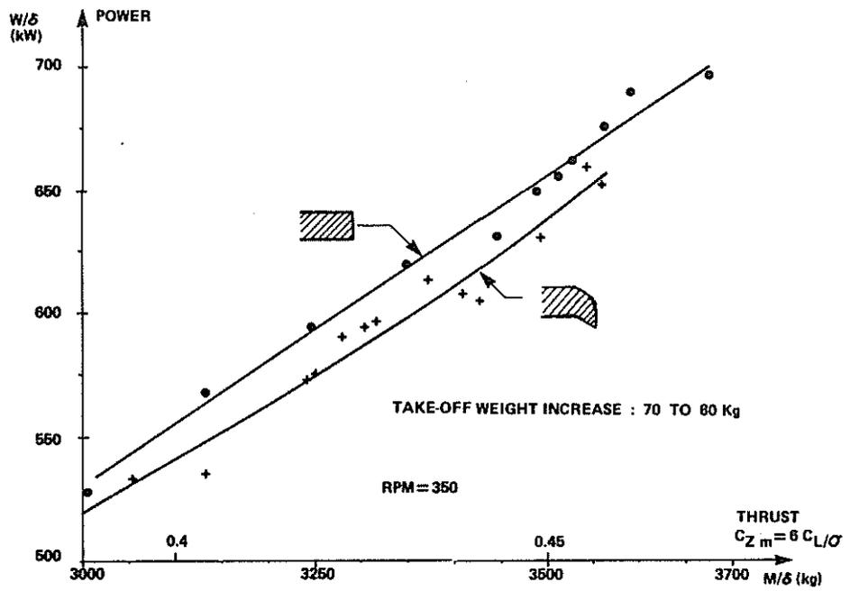
Fig. 7 MAIN ROTOR PERFORMANCE COMPARISON IN HOVER
