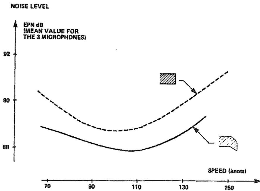
Fig. 18 **REDUCTION OF THE HELICOPTER MEAN EFFECTIVE PERCEIVED NOISE LEVEL DUE TO SWEEPBACK PARABOLIC TIP**
