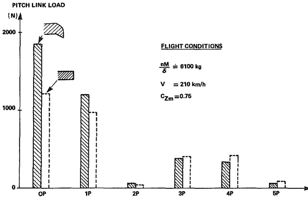
Fig. 14 LOADS ON THE PITCH LINK ROD (STATIC LOAD AND FIVE FIRST HARMONICS)
