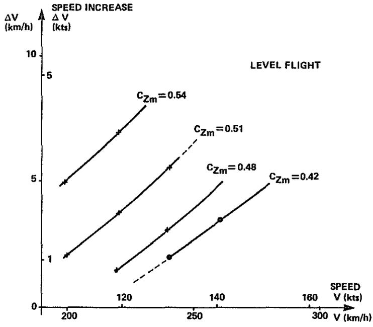
Fig. 11 **SPEED INCREASE DUE TO SWEEPBACK PARABOLIC TIP FOR DIFFERENT VALUES OF THE BLADE LOADING COEFFICIENT (SAME TOTAL HELICOPTER POWER)**
