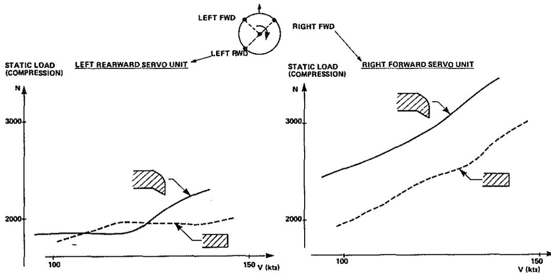
Fig. 13 STATIC LOADS ON SERVO CONTROL UNITS - M=3820 kg
