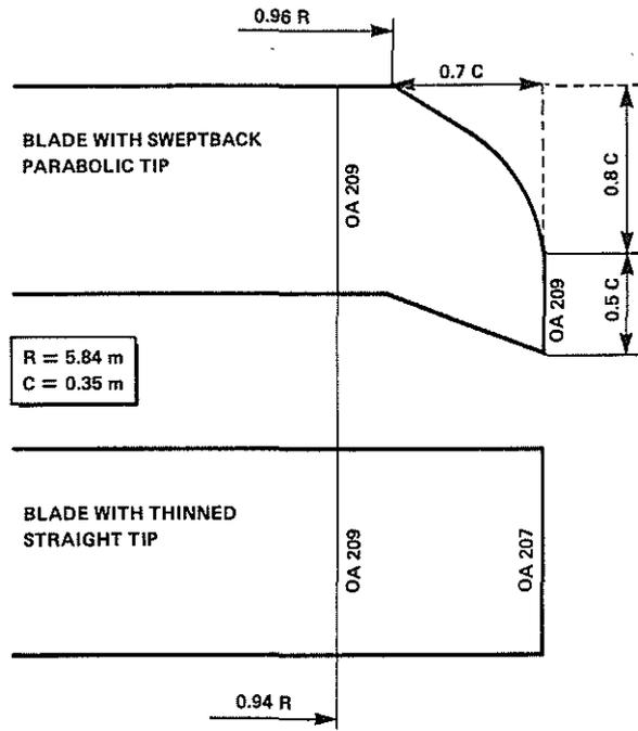
Fig. 5 MAIN ROTOR BLADE GEOMETRY
