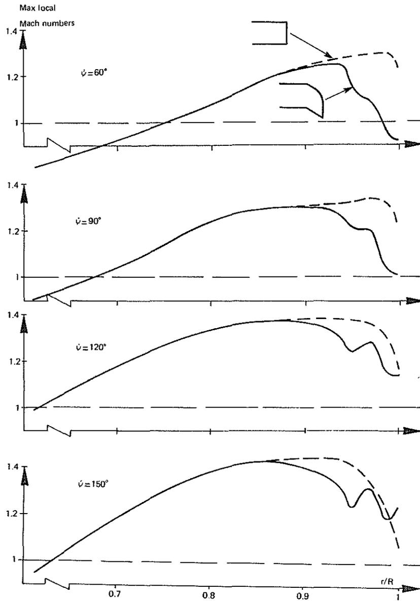
Fig. 18 EVALUATION OF THE MAXIMUM LOCAL MACH NUMBERS ON RECTANGULAR BLADE AND ON BLADE WITH PF2 TIP
