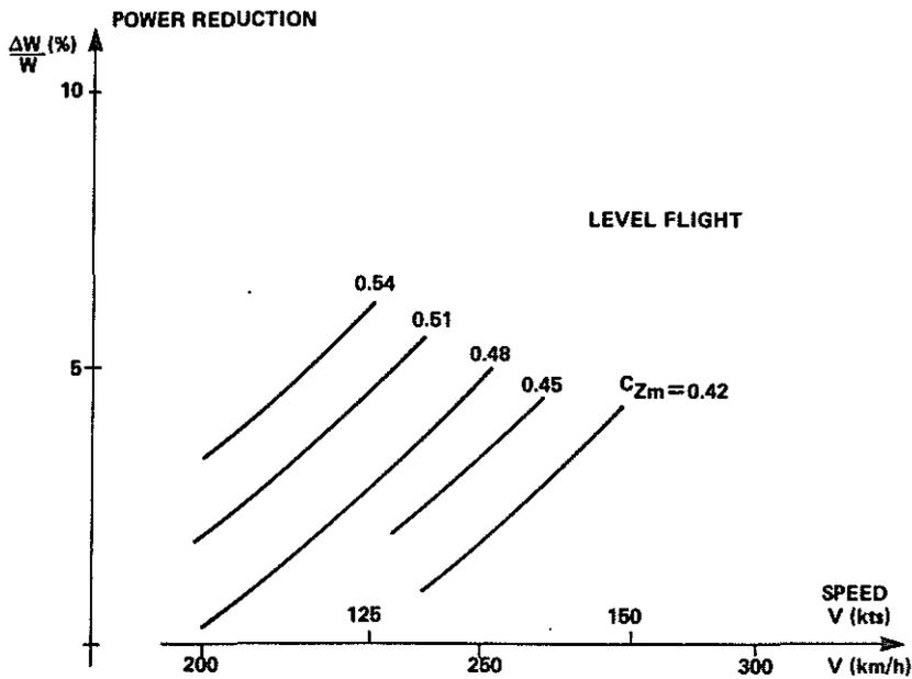
Fig. 10 **TOTAL HELICOPTER POWER REDUCTION DUE TO SWEPTBACK PARABOLIC TIP AS A FUNCTION OF CRUISE SPEED FOR DIFFERENT VALUES OF BLADE LOADING COEFFICIENT**
