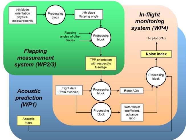
Figure 2: The MANOEUVRES in-flight noise estimation concept.
