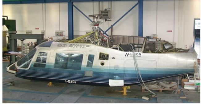
Figure 5: Agusta A109MKII ironbird in the laboratories of the Department of Aerospace Science and Technology, Politecnico di Milano.
