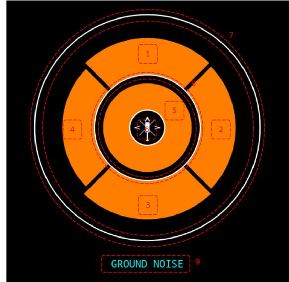
Figure 7: PAI directional indicator: 1 – front sector, 2 – right sector, 3 – back sector, 4 – left sector, 5 – lower sector, 6 – helicopter symbol, 7 – full scale value circle for radial sectors, 8 – full scale value circle for lower sector, 9 – operational mode label.
