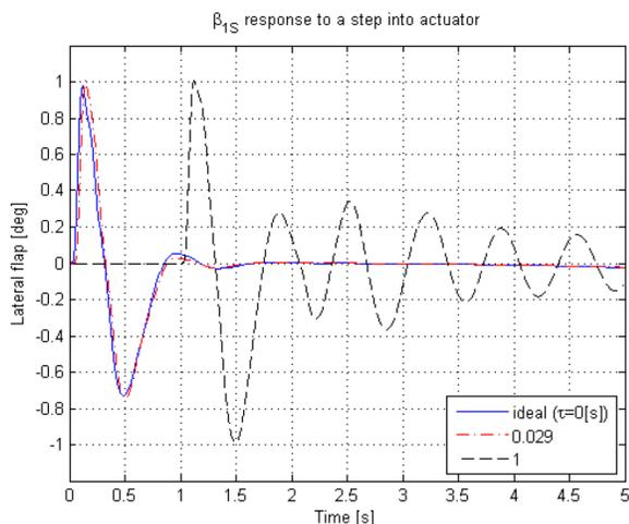
Figure 8: Closed-loop lateral flap response to a step change in the roll angle set point: ideal sensor (blue), realistic sensor (red), low sampling frequency (1 Hz) reference case (green).
