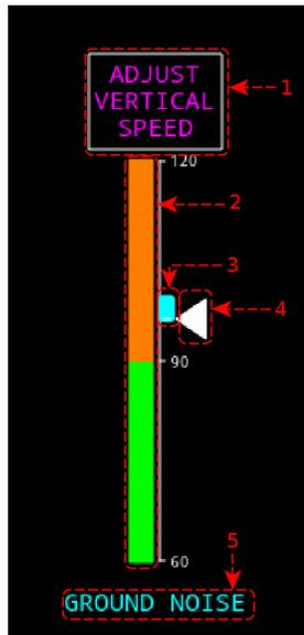
Figure 6: PAI global indicator: 1 – corrective action advice box, 2 – linear scale of the noise index with threshold, 3 – trend bar for the noise index, 4 – current emitted noise index, 5 – operational mode label.
