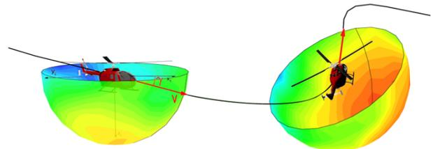
Figure 3: Acoustic emission hemispheric map connected to the manoeuvring helicopter.
