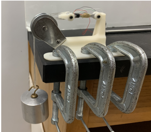
(a) Pitch link calibration of axial load experimental setup
