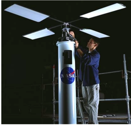
Fig. 3: NASA Ames proof-of-concept Mars rotor hover test stand [2]
