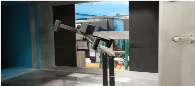
Figure 2: ARL quadrotor vehicle in wind tunnel.
