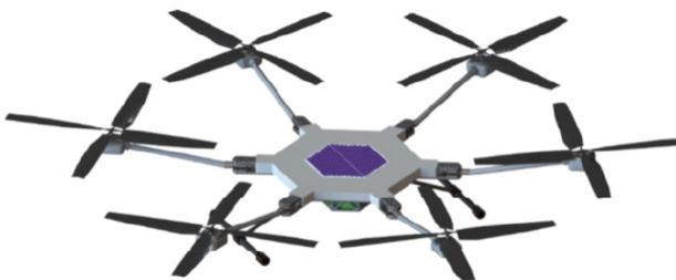
Figure 1: Mars Science Helicopter hexacopter configuration by NASA.
