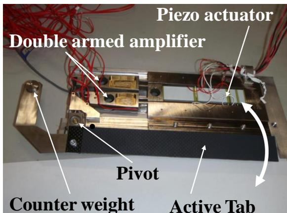
Figure 11: Prototype of Active Tab drive mechanism
