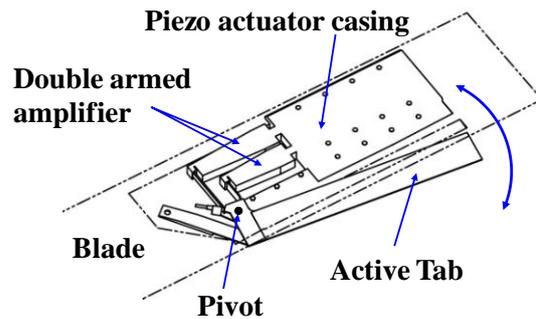
Figure 6 : Drive mechanism of Active Tab
