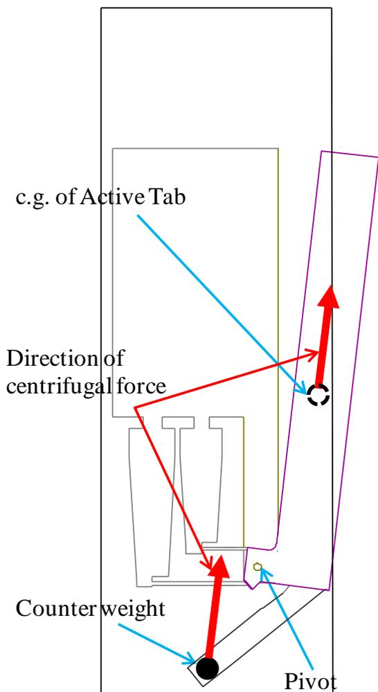
Figure8: Counter weight installation
