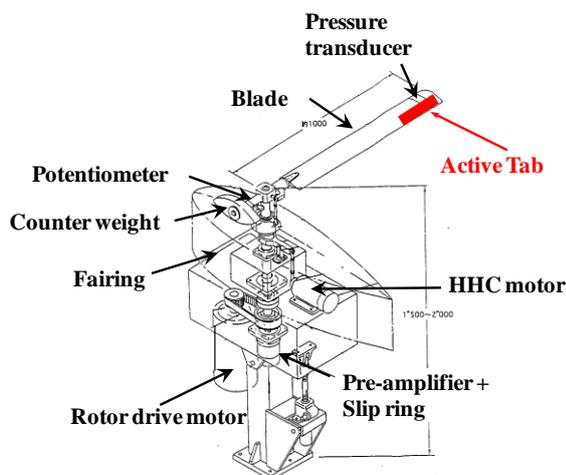
Figure 3: One-bladed rotor system with Active Tab
