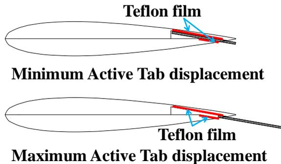
Figure10: Friction reduction measure for Active Tab operation
