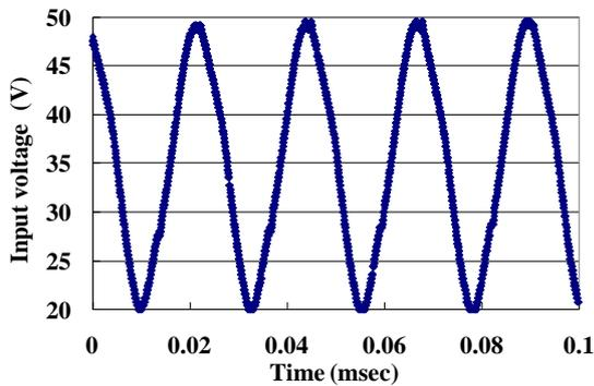
(a) Input voltage to piezo actuator
