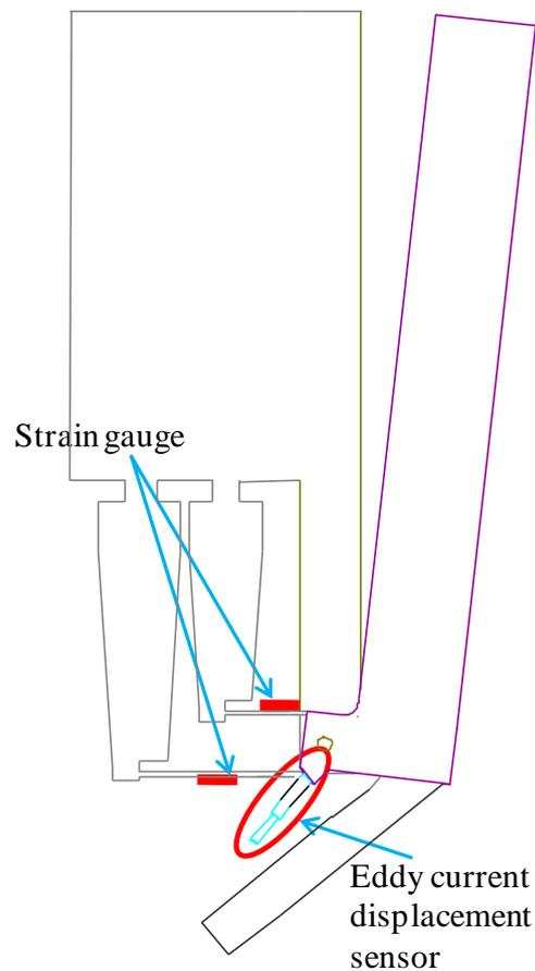
Figure 9: Instrumentation of Active Tab drive mechanism
