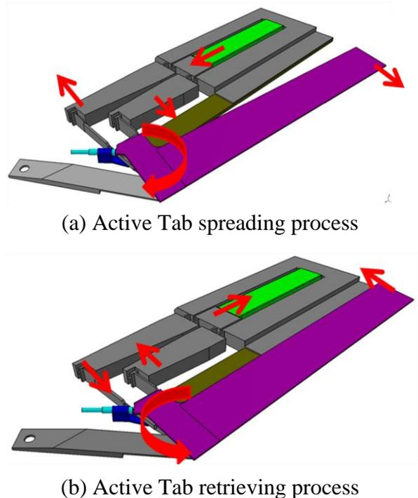
Figure 7: Active Tab deployment sequence
