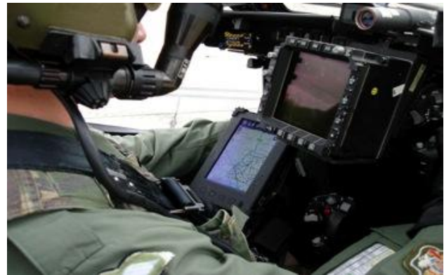
Figure 7: An example of a Knee Mounted Tablet in use in the Apache Cockpit (image courtesy of Inzpire Ltd)
