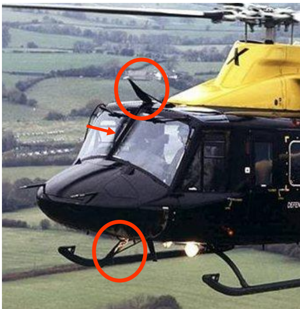
Figure 8: RAF Griffin HT.1 showing wire cutters mounted above and below the cockpit (circled) and deflector on windscreen support structure (arrowed) (image courtesy of www.defenceimages.mod.uk )
