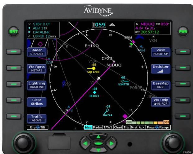
Figure 11: Typical display from Avidyne TAS 615 on EX600 Multi Function Display (image courtesy of Avidyne Corporation)
