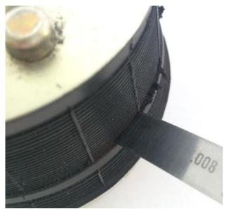
Figure 3: Traditional Crack Depth Inspection Using a Feeler Gage
