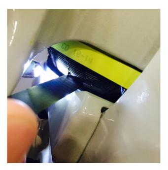
Figure 5: Elastomeric Bearing as Installed on a Helicopter Rotor (Inspection via Feeler Gage)
