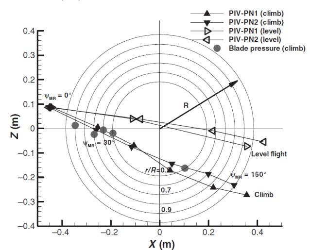
(b) Main rotor tip vortex path across the tail rotor disk, view from port side (wind from left)
