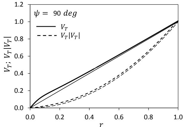
**Fig. 13: Distribution of tangential velocity and dynamic pressure, hover.  $\lambda_{V0} = 0.01$ , vortex in the hub center.**
