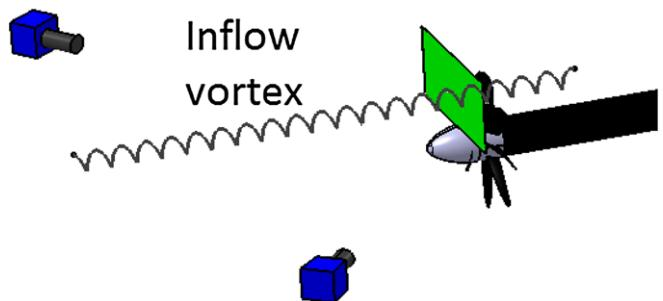
**Fig. 6: Arrangement of vortex-propeller measurements<sup>[13]</sup>.**
