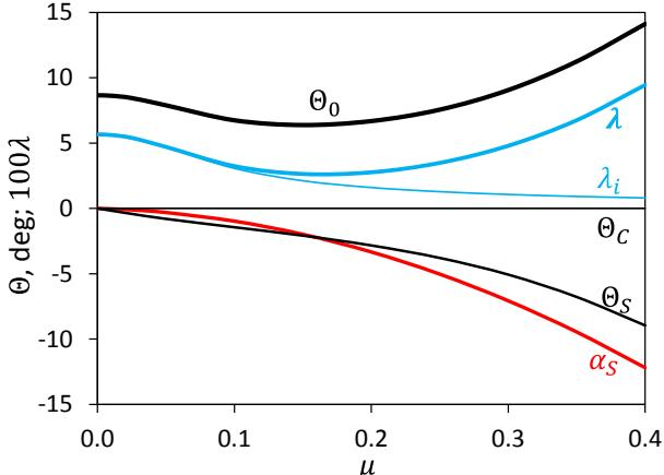
**Fig. 10:** Rotor controls and induced inflow for a trim to constant thrust and zero hub moments.
