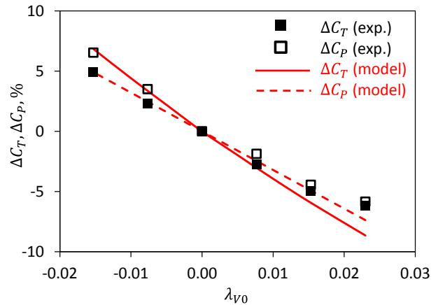
**Fig. 21: Influence of vortex strength and sense of rotation on propeller thrust and power in hover for data from Yang et al.<sup>[13]</sup>.**
