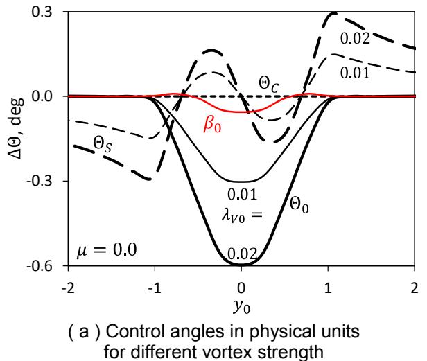
(a) Control angles in physical units for different vortex strength
