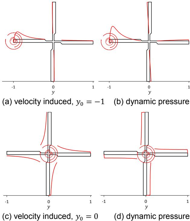
**Fig. 12: Vortex-induced velocities on the rotor blades, hover.**
