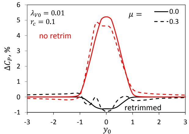
**Fig. 19: Vortex impact on rotor power in hover and forward flight.**
