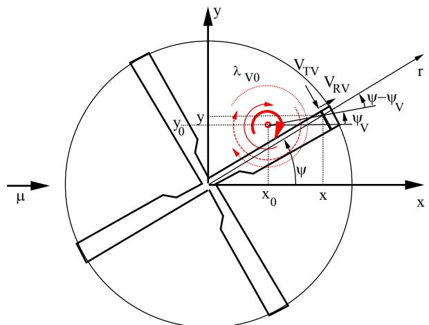
**Fig. 9: Vortex velocities acting at a blade element.**
