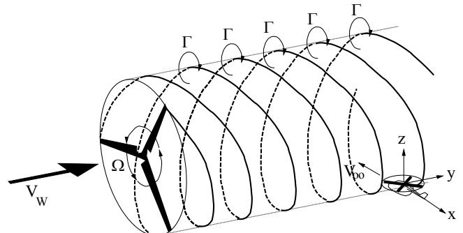
**Fig. 7: Wind turbine wake interaction with a helicopter.**
