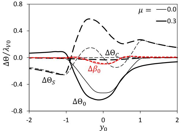
Fig. 15: Controls required to retrim the rotor in forward flight.
