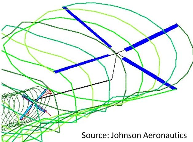
**Fig. 1: Sketch of main rotor-tail rotor interaction.**
