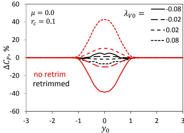
**Fig. 20: Influence of vortex strength and sense of rotation on rotor power in hover.**
