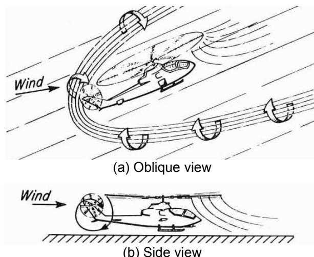
**Fig. 2: Ground vortex-tail rotor interaction<sup>[6]</sup>.**
