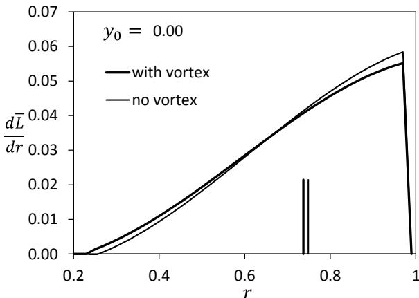
Fig. 14: Lift distribution in hover.  $\lambda_{v0} = 0.01$ , vortex in the hub center.
