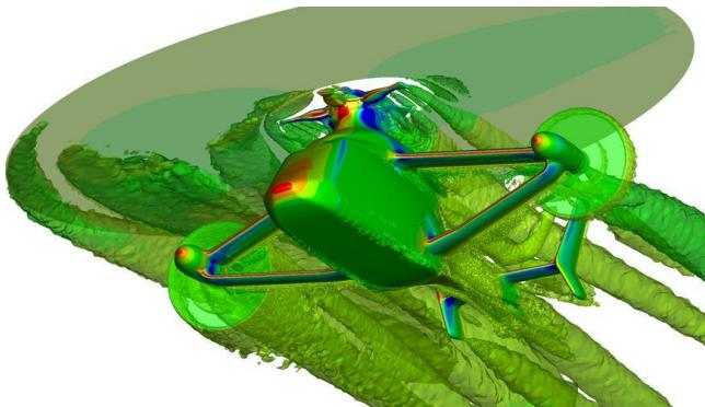
**Fig. 5: Airbus Helicopters Racer box wing design with propellers aft of the wing tips, source: DLR.**
