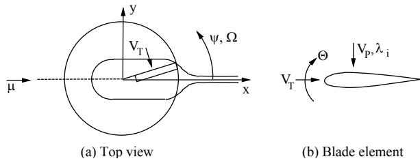
**Fig. 8: Velocities acting at a blade element of a rotor in undisturbed air.**
