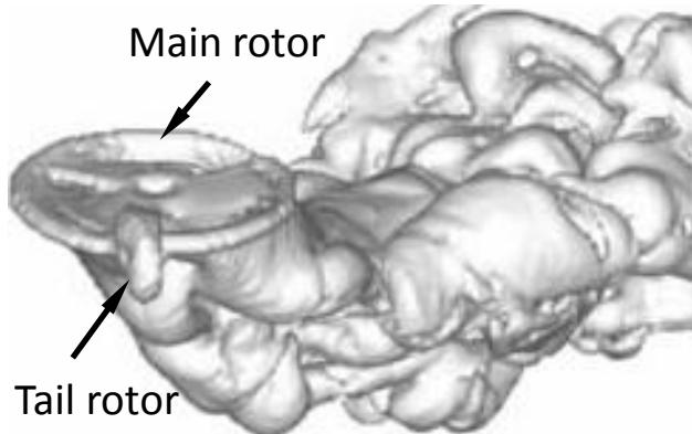
**Fig. 4: Wake structure in quartering flight<sup>[12]</sup>.**
