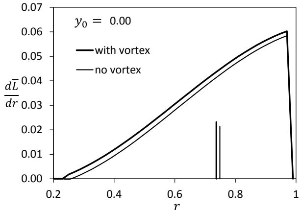
**Fig. 17: Lift distribution without retrim in er.  $\lambda_{v0} = 0.01$ , vortex in the hub center.**
