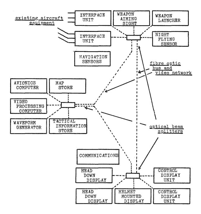
FIGURE 1 Schematic outline of the Inegrated Avionics and Weapon System to be installed in a Lynx Helicopter at Farnborough.
