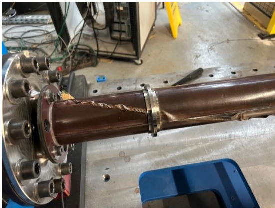
Figure 8: Failure of the shaft 009 in static loading
