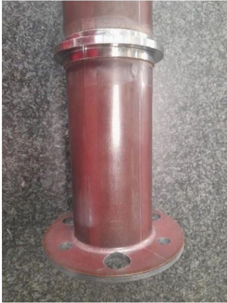
Figure 1: Picture of the tube flange connection of a RECOMPOSE single-piece composite drive shaft
