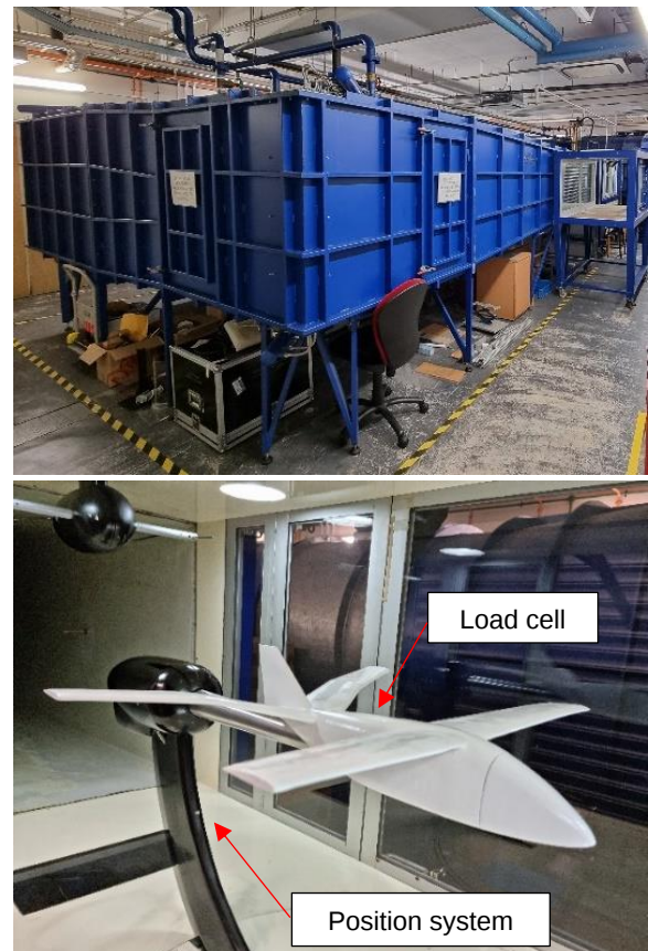
Figure 3: Closed circuit wind tunnel (top), sting position system and load cell (bottom) at NTU.
