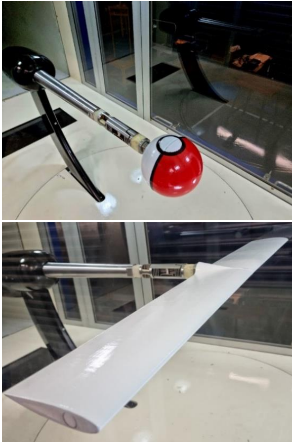
Figure 17: Sphere (top) and NACA0015 airfoil (bottom) used for load cell validation test.
