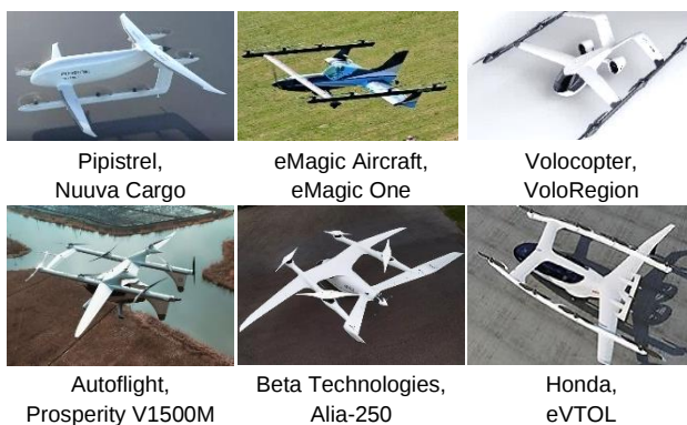
Figure 1: eVTOL aircraft with single long boom design, termed as longitudinal boom mounted rotors.
