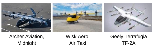
Figure 2: eVTOL aircraft with spanwise distributed rotors, termed as spanwise mounted rotors.
