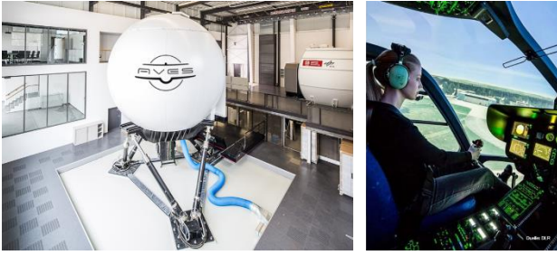
FIGURE 4: The Air Vehicle Simulator (AVES) with its EC135 cockpit at DLR Braunschweig.
