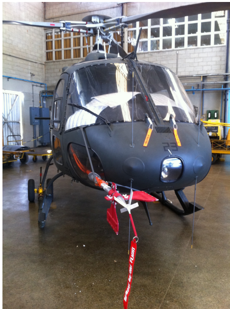
Figure 1 –AS 550 Helicopter with Flight Test Instrumentation installed.
