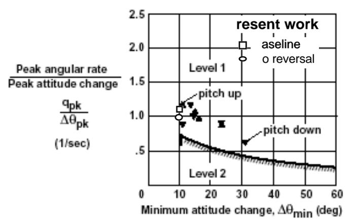
Figure 10: Pitch quickness: comparison with flight test data from Ref. [9].
