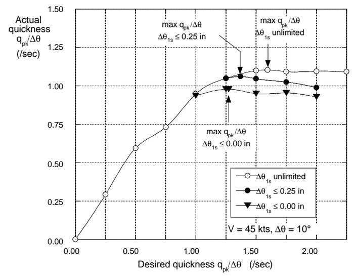
Figure 9: Desired and actual quicknesses for various degrees of allowable control reversal;  $V = 45$  kts,  $\Delta\theta = 10^\circ$ .
