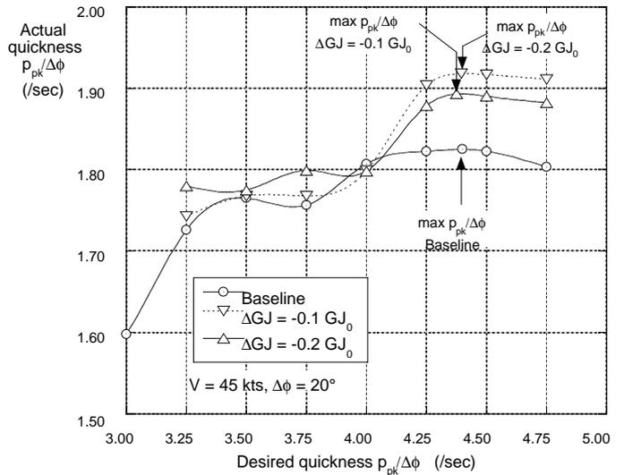
Figure 17: Desired and actual quicknesses for baseline and reduced torsion stiffness blades;  $V = 45$  kts,  $\Delta\phi = 20^\circ$ .
