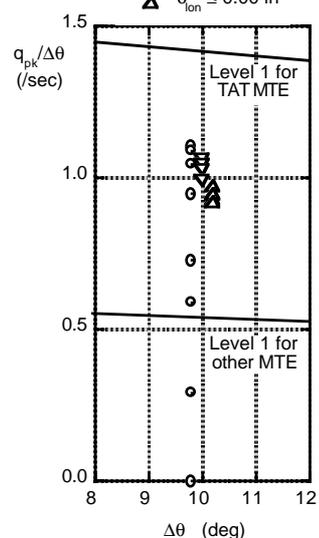
Figure 8: Pilot inputs (top) pitch rates (middle) and quickness (bottom) for various degrees of allowable control reversal;  $V = 45$  kts,  $\Delta\theta = 10^\circ$ ,  $Q_{des} = 1.75$ .
