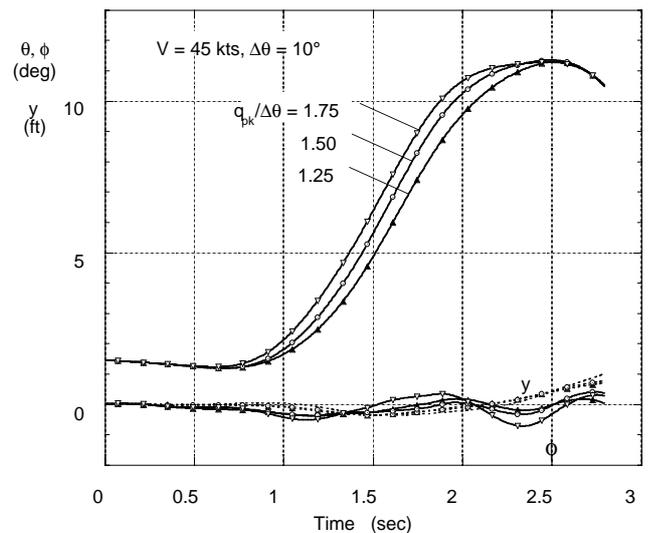
Figure 7: Controls and responses for three actual maneuvers;  $q_{pk}/\Delta\theta$  denotes desired quickness.
