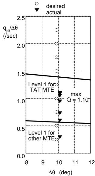
Figure 5: Pitch attitudes, rates, and quickness for desired and actual pitch attitude change maneuvers;  $V = 45$  kts,  $\Delta\theta = 10^\circ$ .
