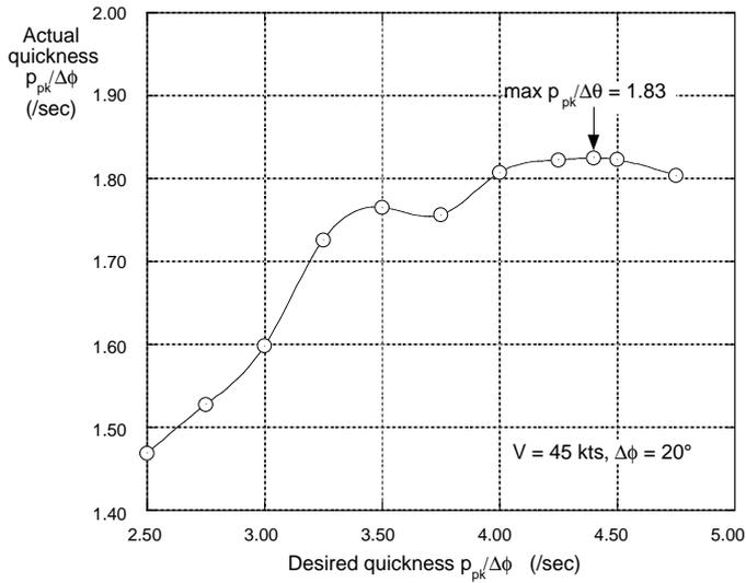
Figure 14: Actual vs. desired quickness in roll attitude change maneuver.
