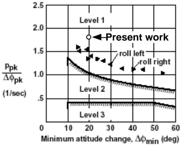
Figure 15: Roll quickness: comparison with flight test data (data from Ref. [9]).
