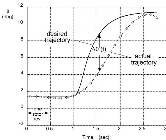
Figure 3: Definition of the optimization-based inverse simulation: example of definition of pilot inputs (top) and of difference between desired and actual trajectory (bottom).
