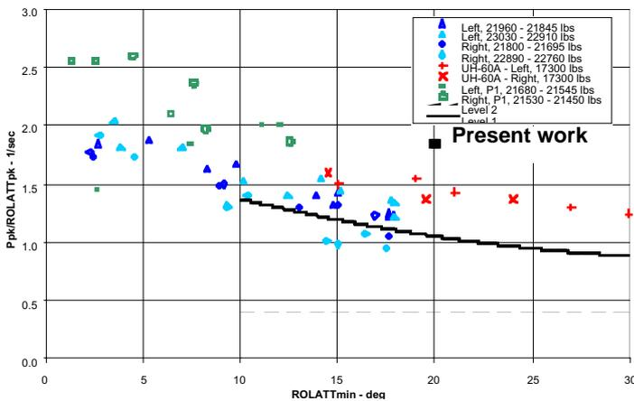
Figure 16: Roll quickness: comparison with flight test data from Ref. [10].
