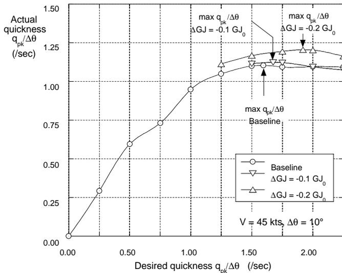
Figure 12: Desired and actual quicknesses for baseline and reduced torsion stiffness blades;  $V = 45 \text{ kts}$ ,  $\Delta\theta = 10^\circ$ .
