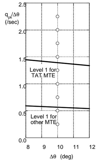
Figure 4: Pitch attitudes, rates, and quickness for desired pitch attitude change maneuvers.
