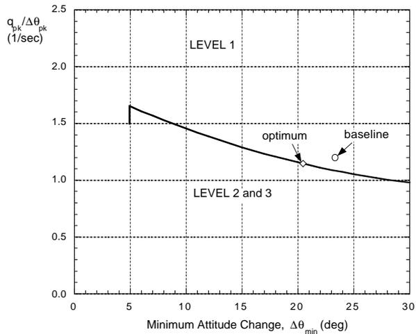
Figure 2: Pitch quickness for baseline and optimized configuration (from Ref. [12]).
