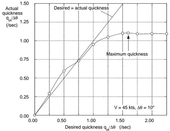
Figure 6: Actual vs. desired quickness in pitch attitude change maneuver.
