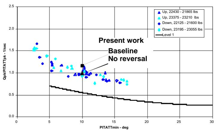
Figure 11: Pitch quickness: comparison with flight test data from Ref. [10].
