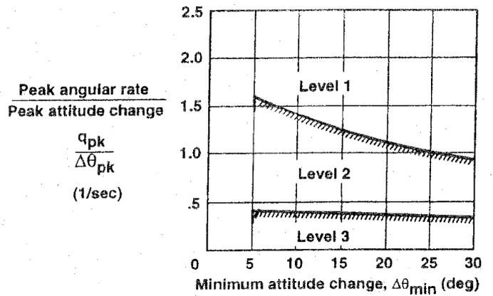
a) Target Acquisition and Tracking (pitch)
