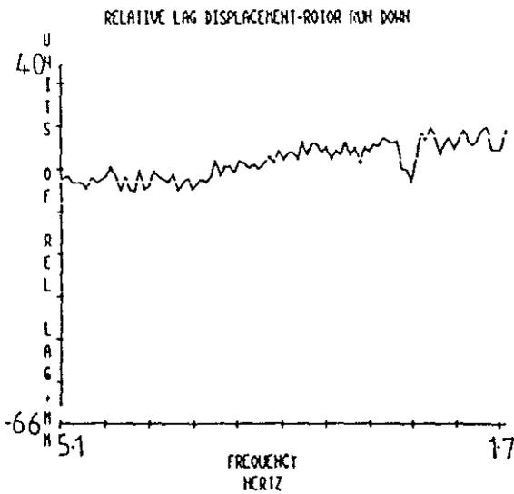
Figure 6. Non steady blade lag trend with an accetable lag damper.
