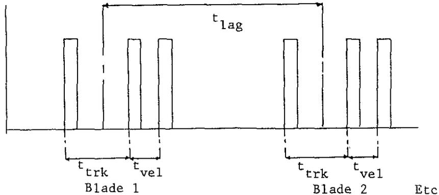
Figure 8. Schematic representation of the blade tracker pulses.
