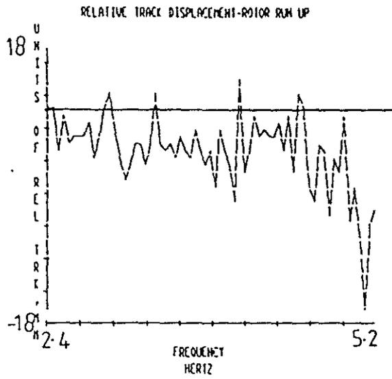
Figure 5. Non steady blade track trend with cumulative tab errors.
