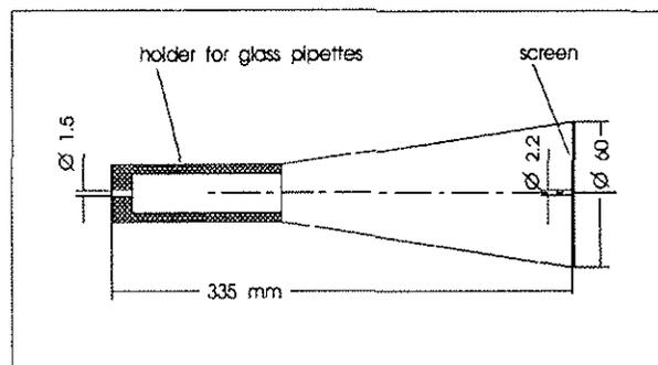
Fig. 2 Flow Visualization Gun - holder for shooting elements
