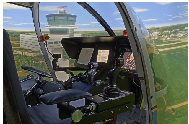
Figure 3: DLR fixed base helicopter system simulation with active side sticks used for the study
