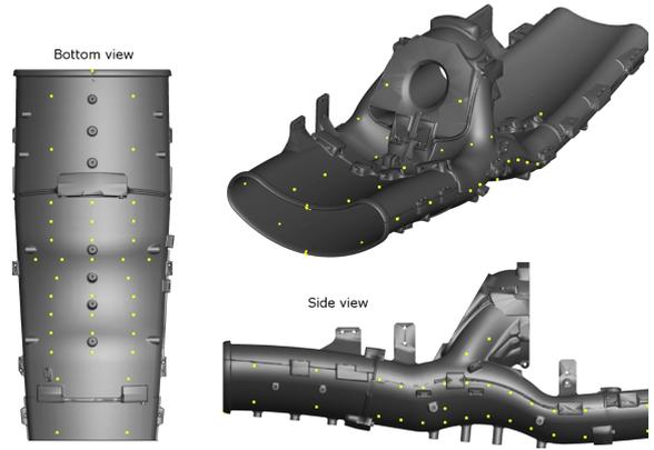
Figure 11: Static pressure taps distribution.
