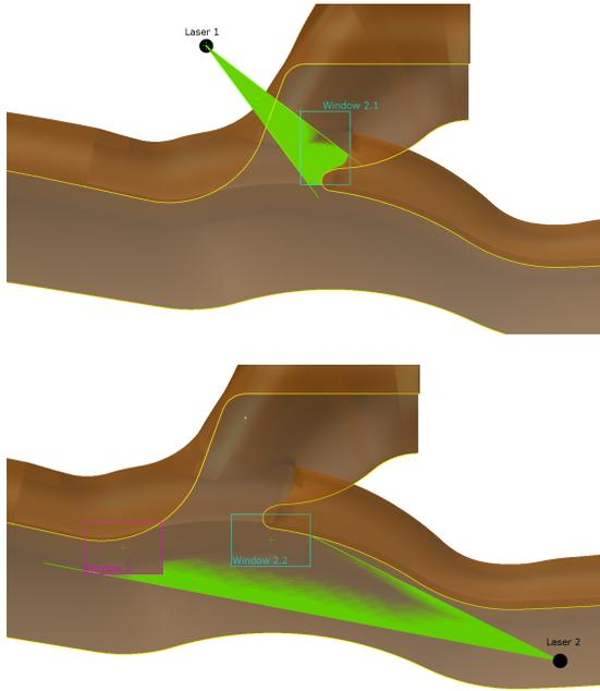
Figure 14: Detail of the PIV field of view.
