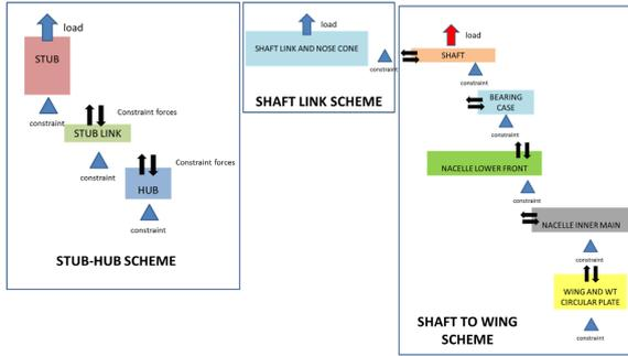
Figure 8: Structural analysis scheme.
