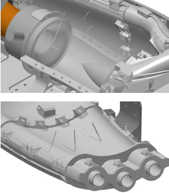
Figure 10: Total pressure probes for flow rate measurement.
