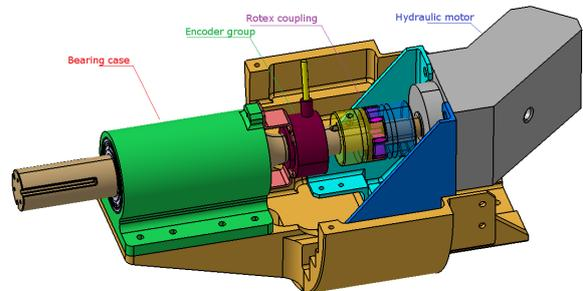
Figure 7: Drive and transmission system.
