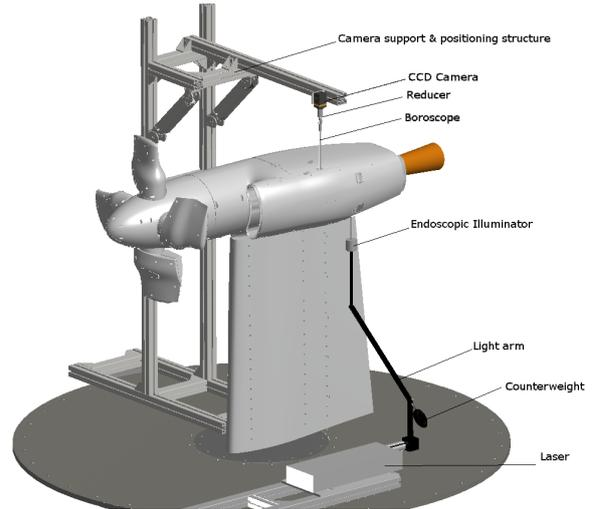
Figure 13: PIV instrumentation layout.
