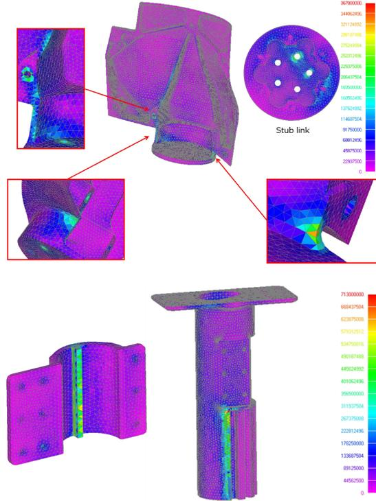
Figure 9: Von Mises stress analysis.
