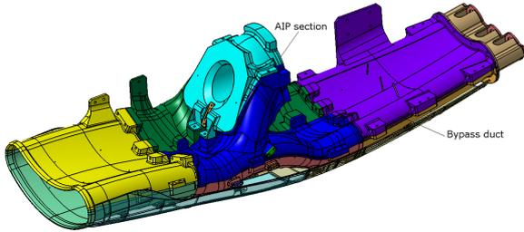
Figure 4: Intake duct model.
