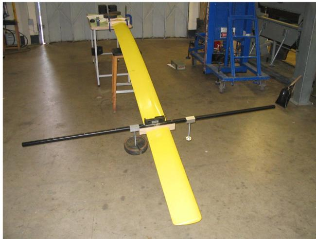
Figure 12 – Arrangement of the experimental measurements of EA position and torsional stiffness of the blade.
