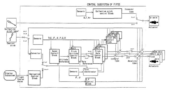
Figure 5. Block diagram of control subsystem
