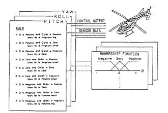
Figure 4 Rate control block
