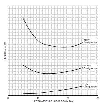
Figure 5 - Height Loss vs Initial Pitch Attitude Delta
