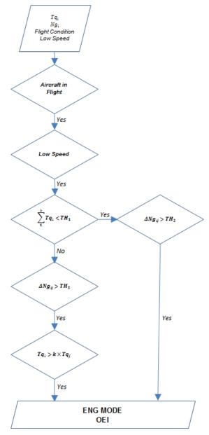
Figure 4 – AFCS Engine OEI Algorithm
