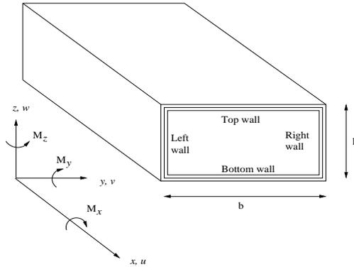
Figure 1. Composite box beam
