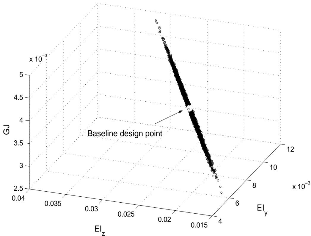
Figure 3. MCS of cross sectional stiffness ( non-dimensional )
