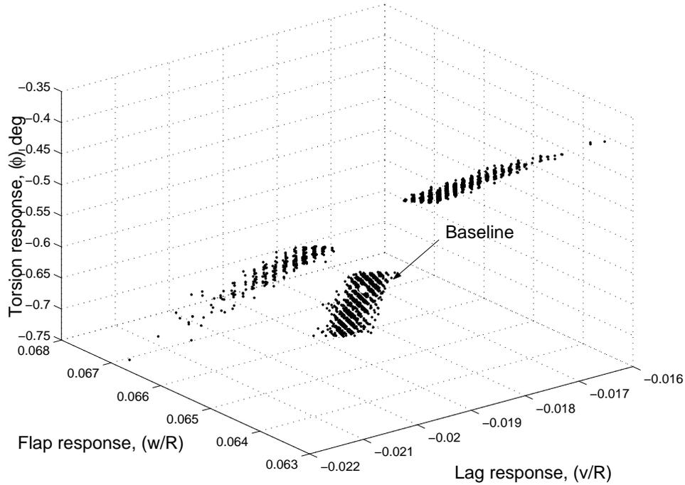
Figure 7. MCS of rotor blade response in hover
