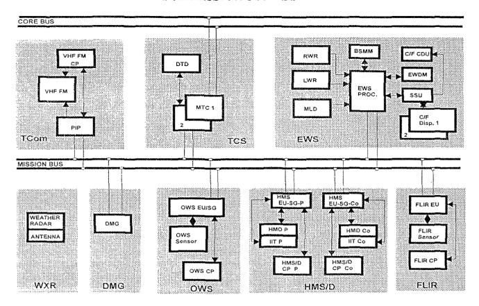
The TMS communicates with the Core System via the CORE Bus, video lines, and dedicated lines.
