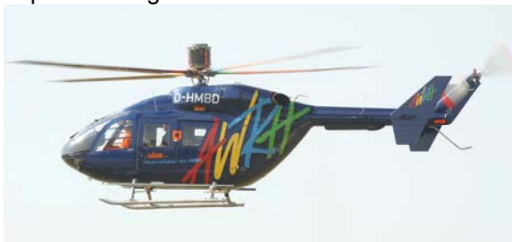
Figure 5: First flight of the BK117 S7045 with active trailing edge flaps
