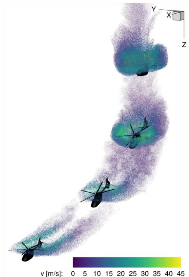
Figure 9: Flight path of the Power-assisted recovery method on a BK117 D-3
