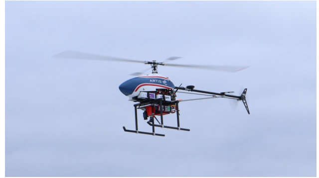
Figure 1: The MIDIARTIS flight test vehicle
