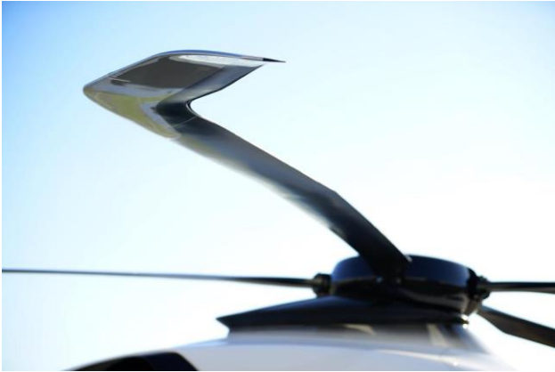
Figure 17: the distinctive double swept shape of the Blue Edge blade equipping the H160 rotor.
