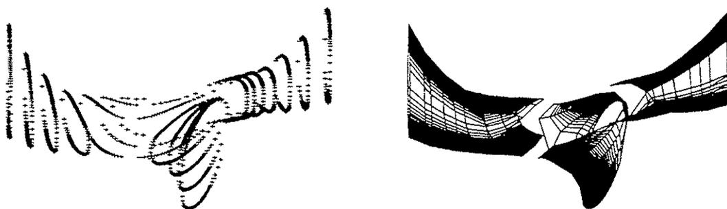
Figure 5 - The panel reconstruction as computed through a linear and three dimensional interpolation, fixing 100 nodes on the different grid layers. The retarded surface refers to a hovering rotor blade at  $M_{tip} = 0.9$ , at one of the highest acoustic emission times.
